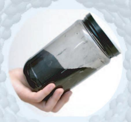
Following the research studies performed by the American Rensselaer Polytechnic Institute, which obtained the darkest material ever made by man (reflective index 0.045 % - 150 times less than conventional black paint) with a thin coating composed by vertically-aligned Carbon Nanotubes, Grado Zero Espace dispersed a low amount of CNTs and micro sized fillers mixture into some polymeric matrices.
